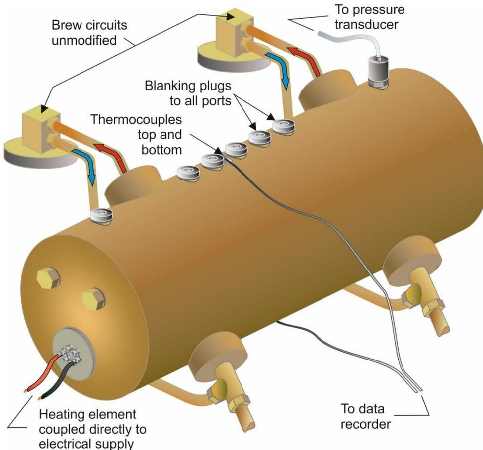
**Figure 3 Instrumentation locations and boiler modifications for overpressure testing**
