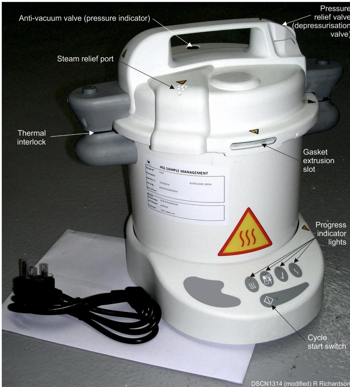
**Figure 58 Benchtop autoclave, features noted in brackets denote secondary function**
