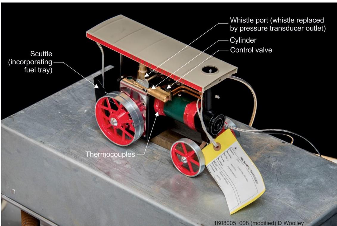
**Figure 69 Miniature Steam Tractor (new model 14424), prepared for testing**
