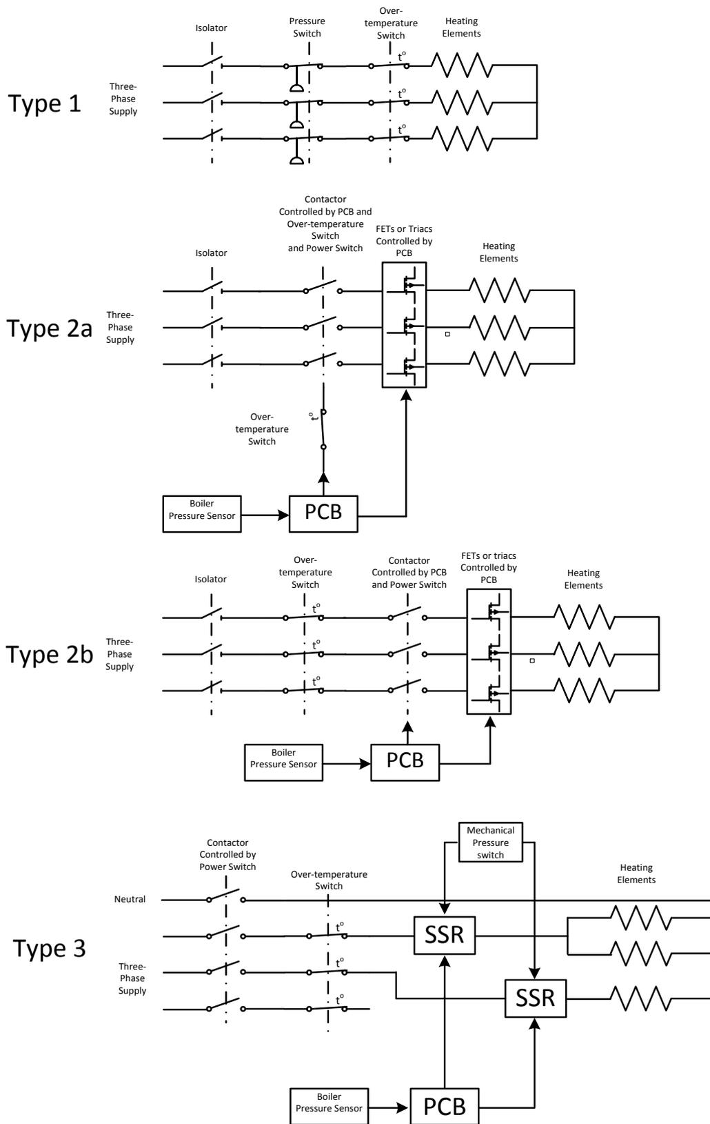
**Figure 2 Control type number schematic**
