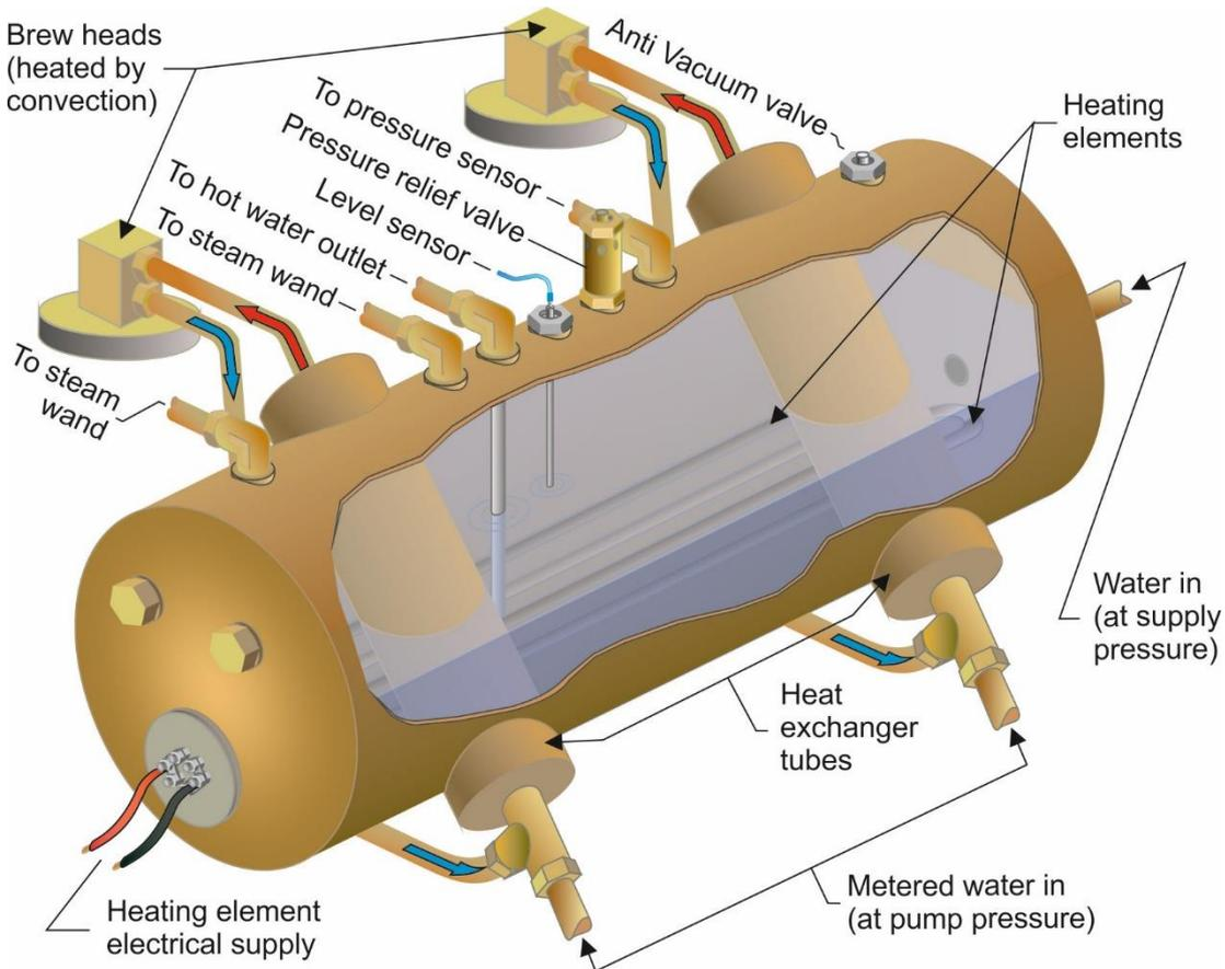
**Figure 1** Cut-away view of a typical café boiler in a two-group professional machine
